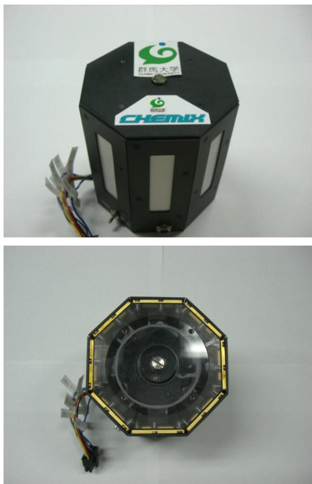
Fig. 5. Pictures of the fabricated passive DMFC stack.
